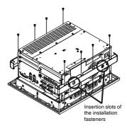
Tight the four provided installation fasteners on the top and bottom of the PL. Be careful for the insertion slots location of the fasteners. The torque required to tighten these screws is 0.8 N·m.
